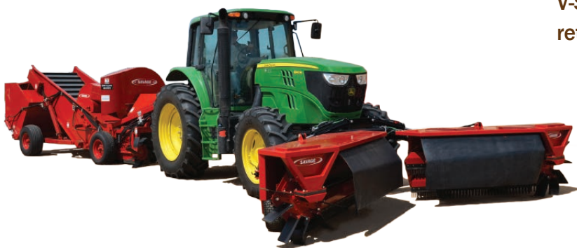
V-Sweeper mounted in tandem with Savage 8548 Row Harvester
